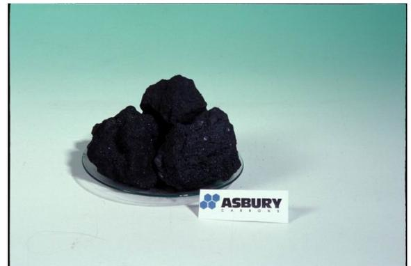
Once removed from the kiln the coke is cooled and routed to whatever application it is destined for. The accompanying photo is of a sample of calcined petroleum coke. Notice that this material has a much higher reflectance than the green coke pictured. Calcined
