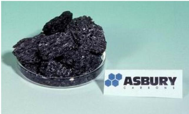
petroleum coke is virtually free of the hydrocarbons which result in lower reflectance. Calcined petroleum coke similar to the material pictured here is the type of coke used as feedstock to make synthetic graphite.
