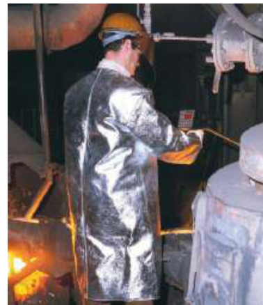
The DL4M instrument being used to take a reading in an induction furnace
